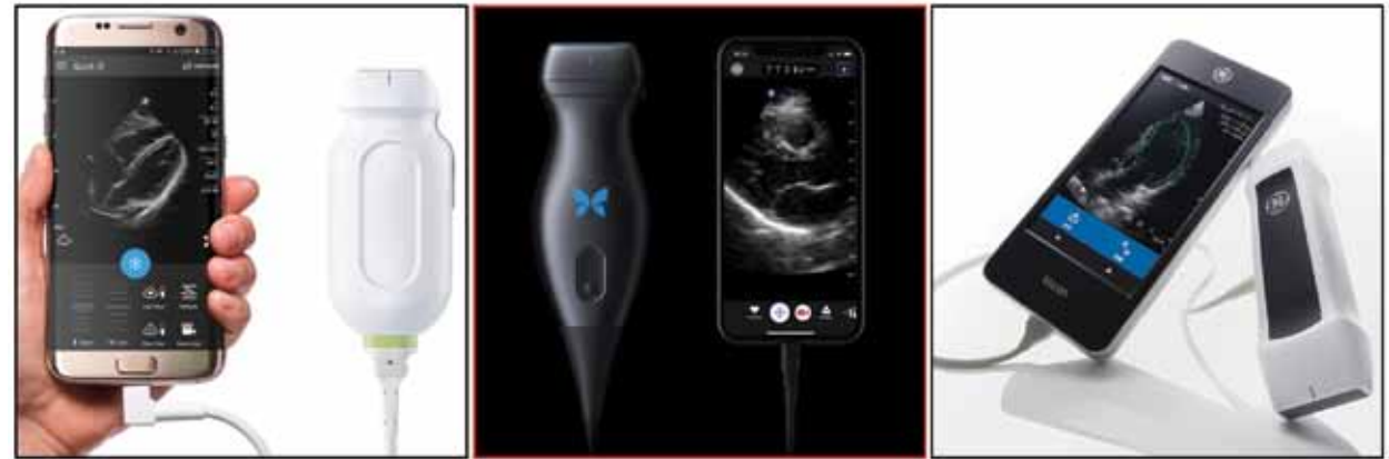
Figure 1. Examples of pocket echo devices. Given their relatively low cost, these devices have potential to be used not only in high-income but also in resource-limited countries. In a perfect world, most clinicians should have one in their pocket and be trained for basic qualitative ultrasound evaluations. From left to right: Lumify from Philips, IQ from Butterfly, VScan from GE Healthcare.
