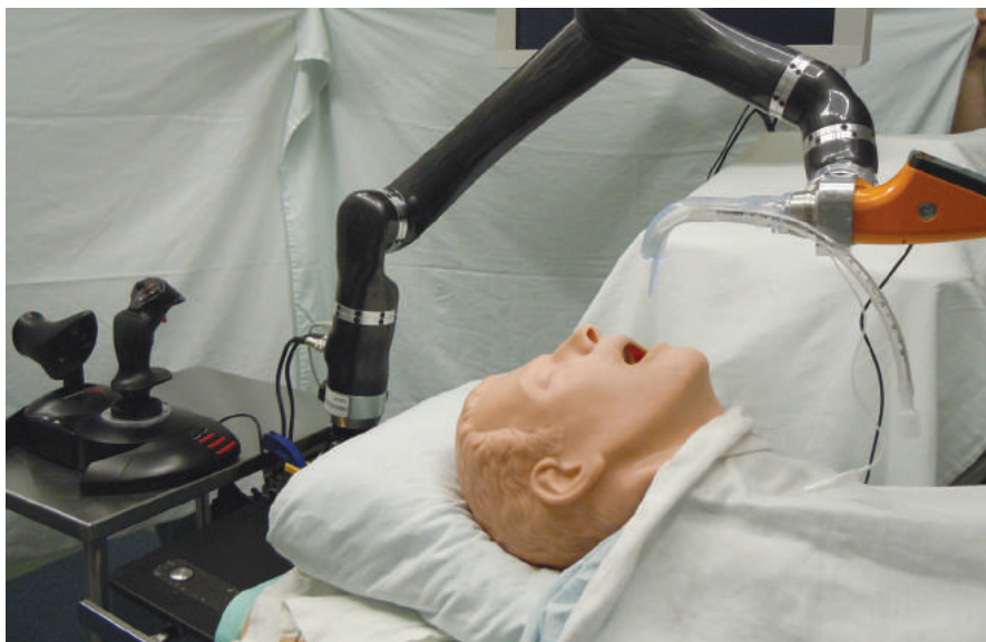
Figure 2. The Kepler Intubation System. The robotic arm is able to move into the 3 spatial plans, imitating the movements of arms and wrists. A camera is placed on it for live video feeding. On the left: the joystick.
