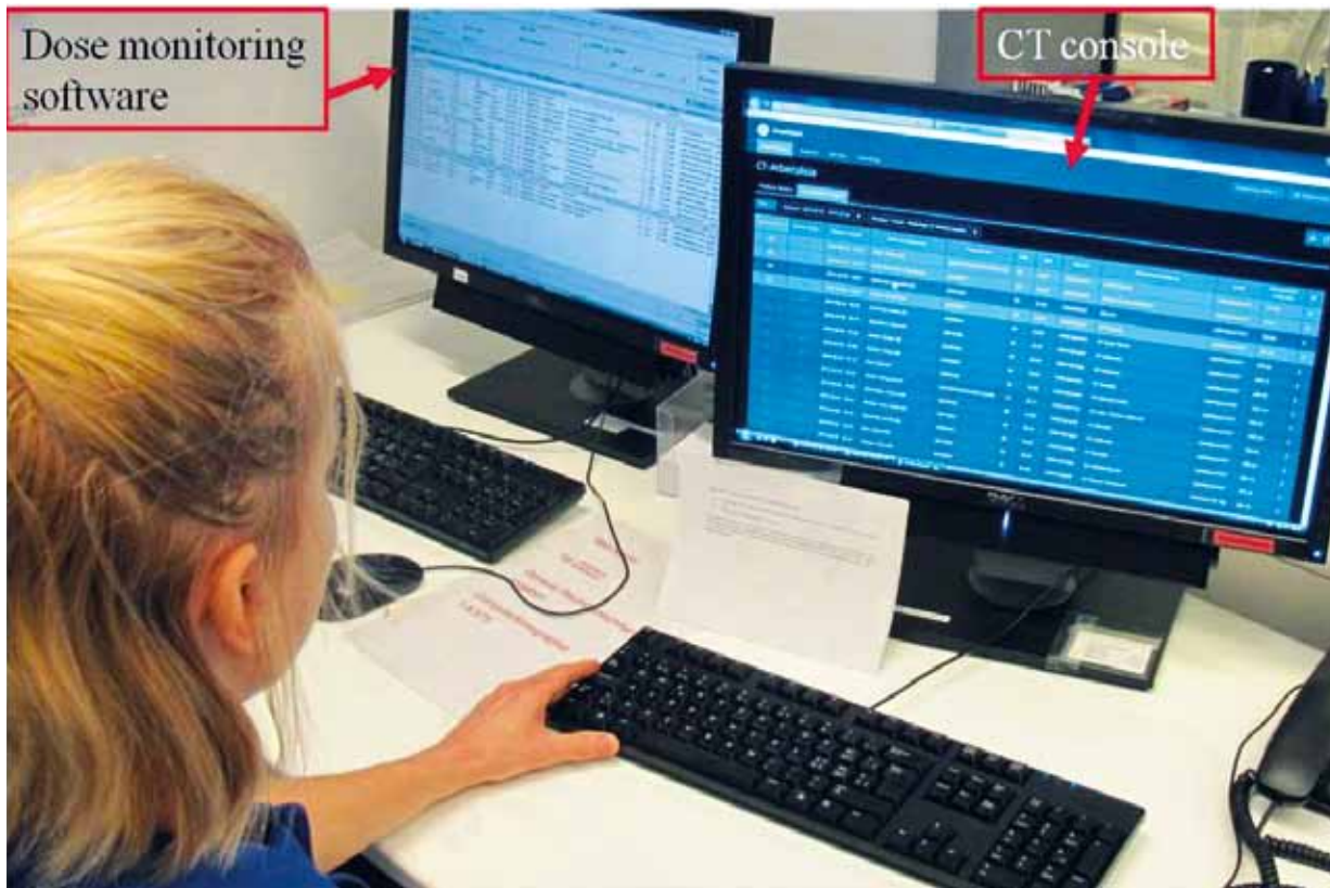
Figure 2. An additional computer with the dose monitoring software permanently running was placed next to the CT console to assist dose control and support dose culture.
