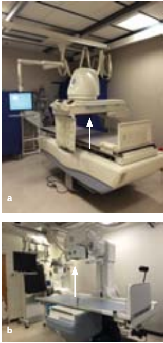
Figure 1. Images Comparing Fluoroscopy Equipment Figure 1a - Industry standard fluoroscopic machine has a table weight limit of 350 lbs [158kg] and 18" [45.7cm] aperture (white arrow). Figure 1b - Bariatric fluoroscopic equipment has a table weight limit of 500 lbs [226kg] and aperture opening of 44" [111.7 cm] (white arrow).
