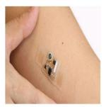
Engineers at the US University of Illinois and Northwestern University have showcased soft stick-on patches thin enough to move and stretch with the skin, and equipped with chip-based electronics for latest technology enabled wireless health monitoring. The researchers have published their design in the April 4 issue of 'Science'.
