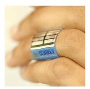
University of Surrey researchers have developed a new flexible x-ray detector that they claim can achieve high sensitivity levels that strongly compete with current technologies. The researchers also proved that it is possible to create a device that conforms to the subject – i.e., it could be possible for breast cancer screenings to be carried out by adapting the x-ray detector arrays to the specification of different patients. This functionality is not available with current x-ray detectors.
