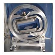
Researchers from Imperial College London have developed a prototype for a 'mini' MRI scanner specifically to fit around a patient's leg.
