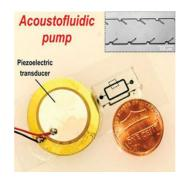
Bioengineers and scientists at Pennsylvania State University have developed an acoustofluidic pump that is powered by a piezoelectric transducer. The pump utilises the acoustic streaming effects generated by the oscillation of tilted sharp-edged structures that are hundreds of micrometres in length and that are constructed onto the sidewall of a microfluidic channel made of polydimtehylsiloxane (PDMS).
