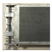
Scientists in the U.S. added a collimator to an existing 3-D breast molecular imaging system that improved image quality in the contrast of cancer lesions in the breast and slashed the radiation dose to the patient by half.
