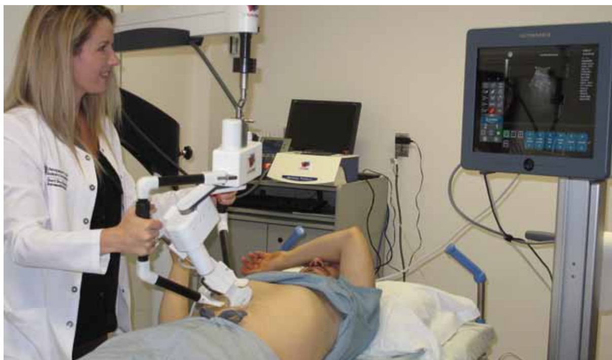
Figure 1. A remote clinic is equipped with an ultrasound unit and robotic arm (MELODY Patient System, AdEchoTech, Naveil, France) to which an ultrasound transducer is attached. An assistant with no prior ultrasound experience guides gross placement of the frame for the robotic arm based on instructions from the sonographer or radiologist.
