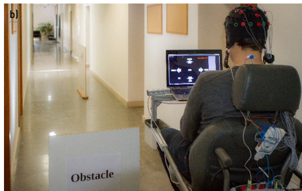
Figure 4: a) Robotic hand for neurorehabilitation combining EMG and EEG; b) A BMI system used to control a wheelchair (Cruz et al. 2021).
