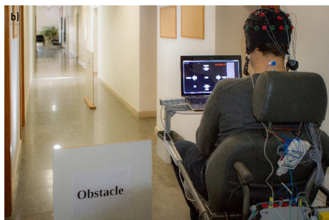
Figure 4: a) Robotic hand for neurorehabilitation combining EMG and EEG; b) A BMI system used to control a wheelchair (Cruz et al. 2021).
