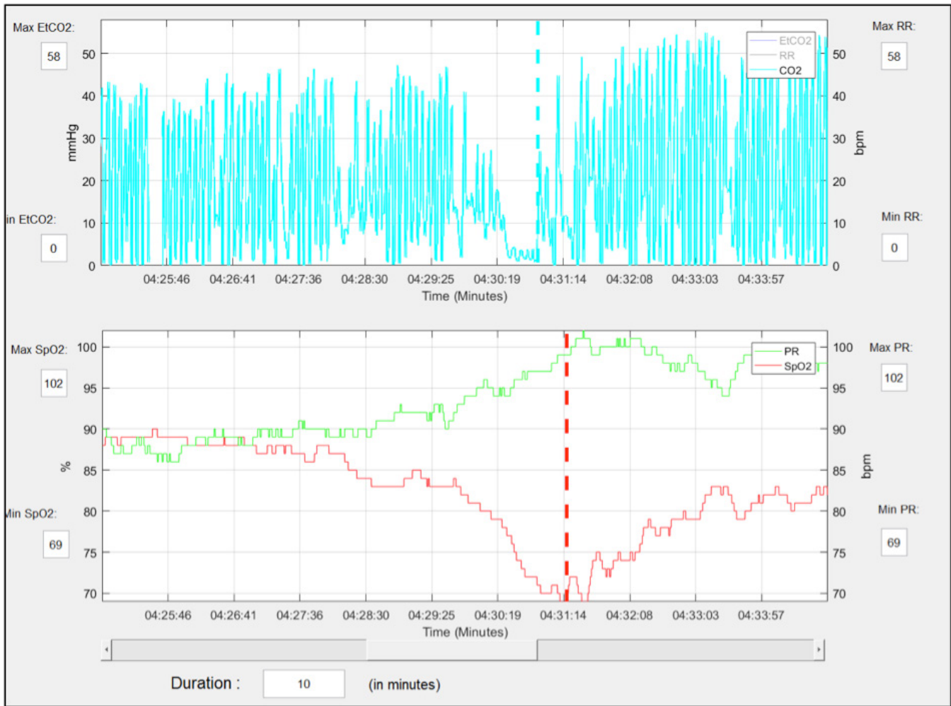
Figure 2. Data from the PRODIGY trial showing continuously monitored capnography and oximetry data showing a significant apnoea hypoxaemia episode (blue and red dashed areas)
